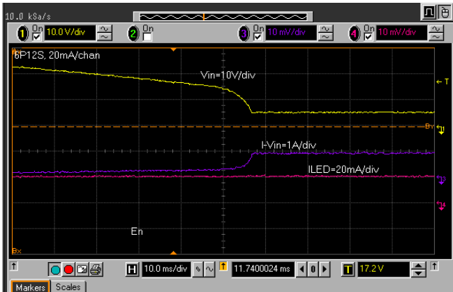
FIGURE 15. LINE REGULATION WITH V_{IN} CHANGE FROM 26V TO 6V FOR 6P12S AT 20mA/CHANNEL
